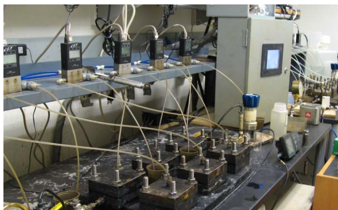
Figure 1: Flat-sheet Cell Testing Bench
