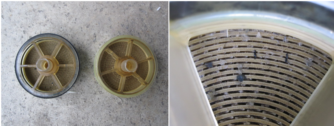
Figure 7: End caps. Feed on left, brine on right Figure 8: Close up of feed endcap
